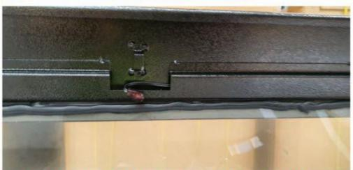
Image shows IR repeater dragged through enclosure channel and places in the middle of the enclosure lid facing outward.
